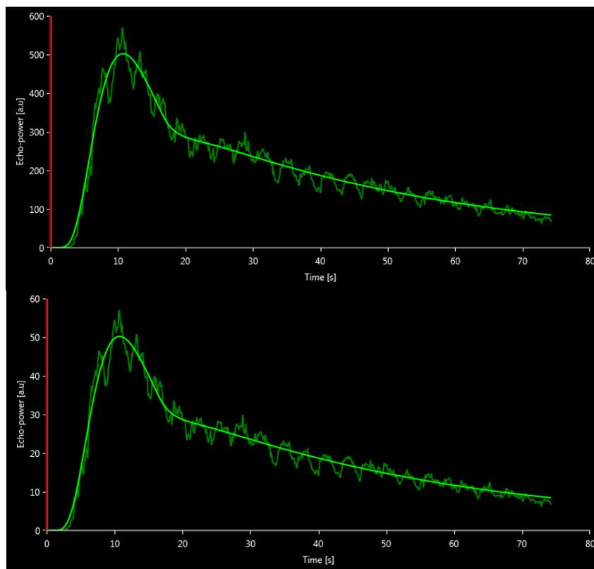
**Figure 13 - Example of signals before and after gain compensation. In this case, we needed to compensate for a gain of 10 dB, meaning a compensation of -10 dB should be applied. Therefore the amplitude of the signal at the end is multiplied by 0.1 ( $10^{-Gain/10}$ ).**
